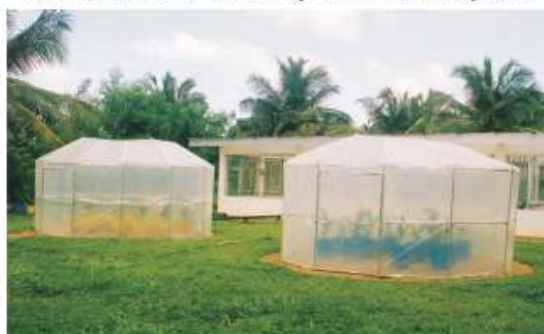
Fig. 3.18. Open Top Chambers (OTC) with coconut seedlings exposed to elevated CO 2 (left) or ambient CO 2 (right).
